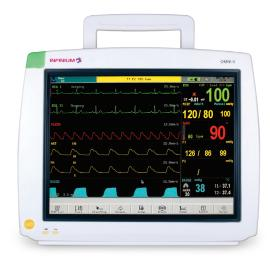
The **Omni II**<sup>™</sup> offers a 3, 5, and 12 lead ECG platform. Arrhythmia detection and ST are also standard and measurable on all lead sets.
